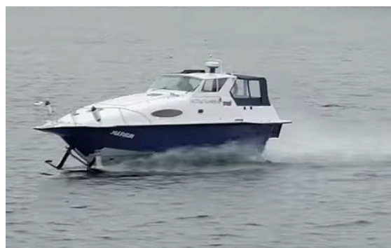
Photo of a prototype vessel with spent hydrodynamics of the hull and up/down foils
