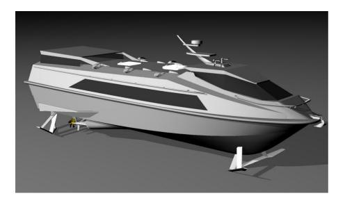
«Alfa" type boats in exploitation (operation) mode are like conventional gliders, but has its fuel consumption (in comparing speed and weight) about twice less then gliders.«Alfa-70" passenger hydrofoil can be delivered full tested and equipped. Boat can be built according Russian or BV classification rules.
